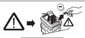
Note: It may be necessary to check if this vehicle has a stored radio code before disconnecting the battery!
